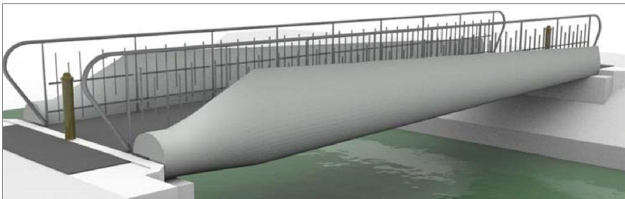
A conceptual design of pedestrian bridge using A29 wind blades as main girders, Re-Wind research project <sup>[24]</sup>
