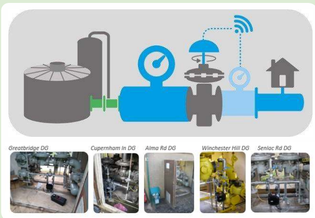
Figure 9-4 Remote pressure control and management
