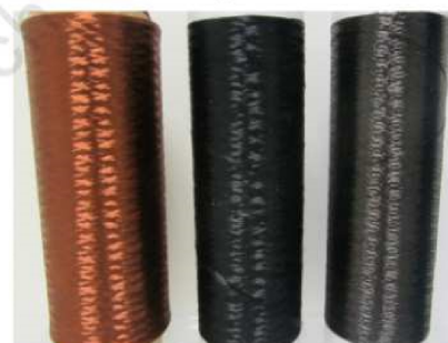
Precursor stabilized fiber carbon fiber
